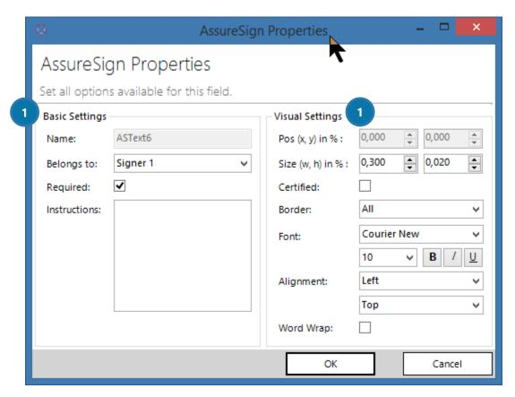
Figure 12: AssureSign Properties-window functionalities (for the Text-type)
